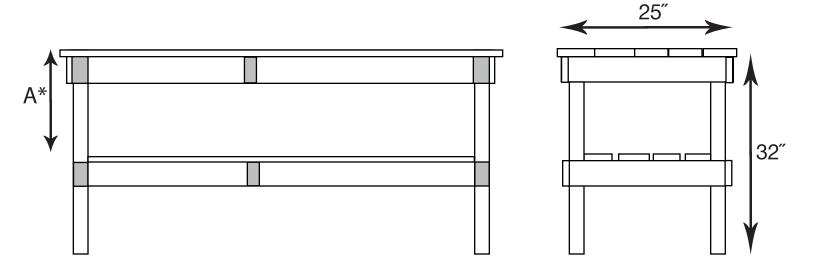
\*A is the measurement from the top of the lower shelf to the top of the table. The A measurement is 10"
